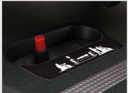
Two-step disengaging lever to prevent free-wheeling
